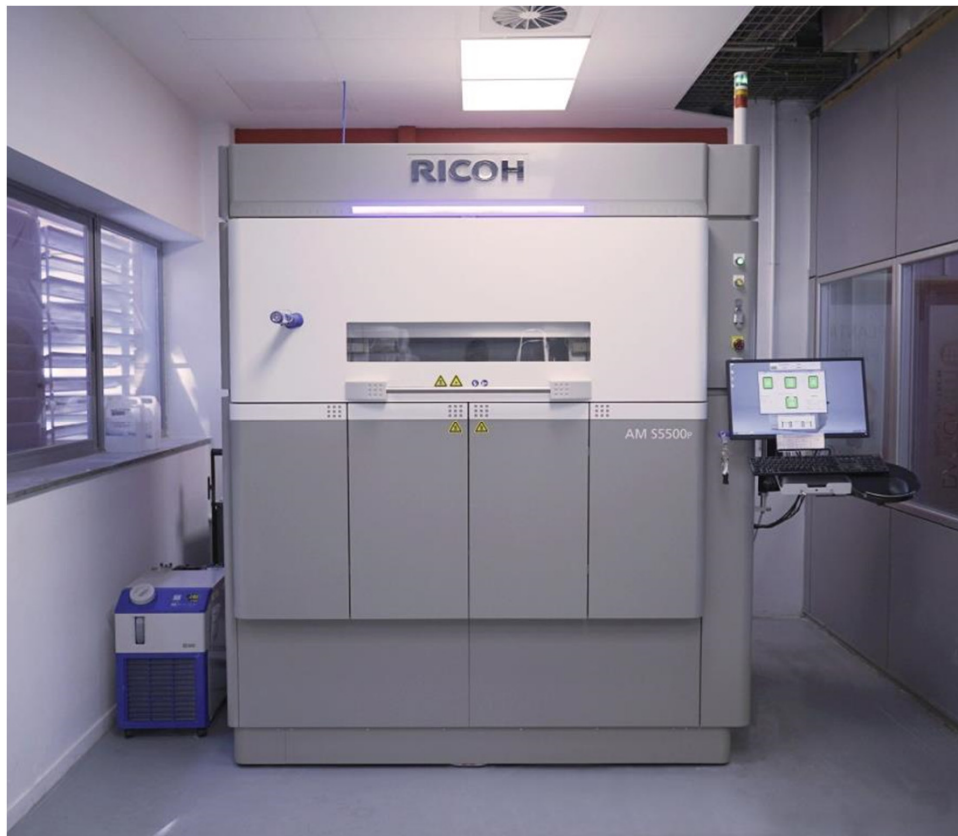
RICOH AM S5500P Powder Bed Fusion Machine located at Ricoh Additive Manufacturing Centre in Barcelona (CIM UPC facilities) . Huge platform, 550x550x600 mm.
